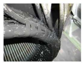
Grey treatment (marinization) on the left, TOTAL+ treatment shown on the right. The EG43 grey varnish, is an high temperature insulating enamel that forms a tough and flexible film, with excellent moisture and chemical protection. It is water and oil proof, and also protects windings from abrasion. It is applied spraying an over coating layer over the impregnated winding, or dipping the stator in a varnish barrel for superior treatments
